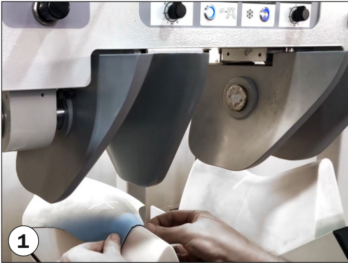
Step 1. Place the vamp in the hot station mould as shown in Figure 1
